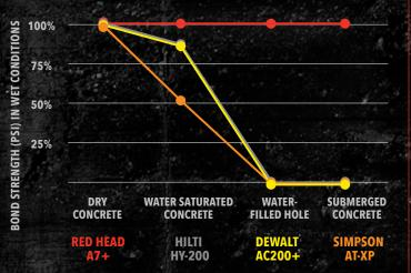
Data taken from evaluation reports listed on www.icc-es.org as of 11/1/17. Based on #6 rebar for uncracked concrete with periodic inspection. The bond strength for each product in wet conditions is represented above as a percentage of the performance of the same product in dry conditions.
