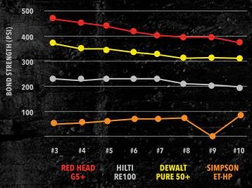
Data taken from evaluation reports listed on www.icc-es.org as of 11/1/17. Based on Rebar in cracked, saturated concrete with periodic inspection.
