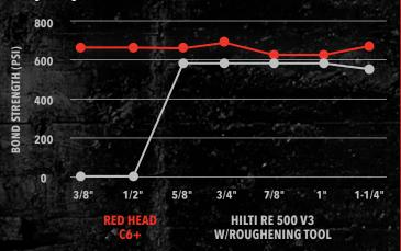
Data taken from evaluation reports listed on www.icc-es.org as of 11/1/17. Based on threaded rod in a coredrilled hole in cracked, saturated concrete, with periodic inspection.
