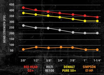
Data taken from evaluation reports listed on www.icces.org as of 11/1/17. Based on threaded rod in cracked, saturated concrete with seismic conditions and periodic inspection.
